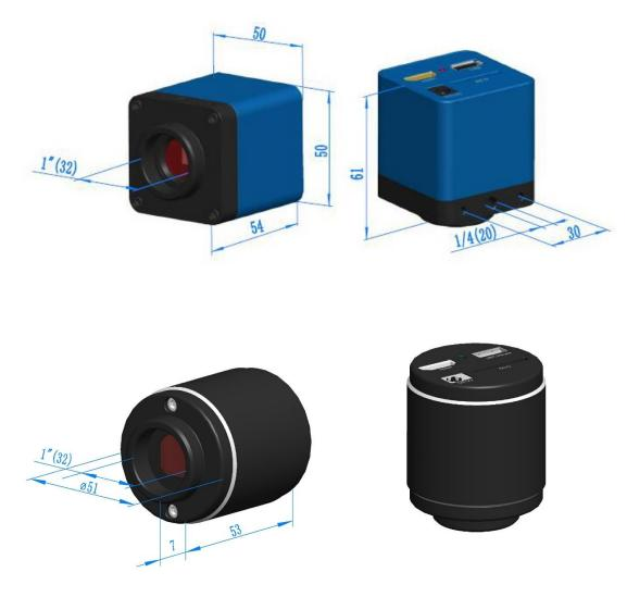
Figure 3-1 Dimension of XCAMLITE1080P Series
