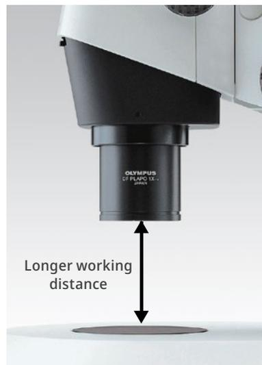
Objective lenses: 1x for task efficiency
