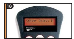
For the second alignment object, choose a bright star or planet as far from the first alignment object as possible. Once again use the directional arrow buttons to center the object in the finderscope and press ENTER. Once object is centered in the eyepiece, press ALIGN.
