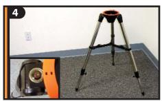
All three legs should be the same length to provide a level platform for the telescope. A bubble level is included (inset) to assist in leveling.
