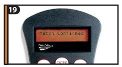
Repeat the process for the third alignment star. When the telescope has been aligned to the final star, the display will read "Match Confirmed". Press UNDO to display the names of the three bright objects you aligned to, or press ENTER to accept these three objects for alignment.
