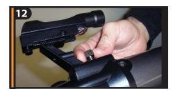
Secure finderscope to mounting platform by tightening the silver screw. The glass window of the finderscope should be facing towards the front of the telescope.
