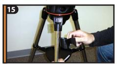
Attach plastic hand control holder to the tripod leg.
