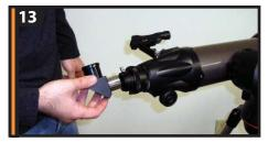
Insert the chrome barrel of the star diagonal into the focuser and tighten the two silver screws to secure in place.
