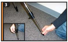
Extend tripod legs 6 to 8 inches by loosening the tripod leg locking knob and pulling the leg to desired length and re-tightening knob.
