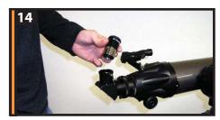
Select the low power (25mm) eyepiece and insert it as shown above. Tighten silver screw to secure.
