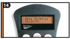
Using the numeric key pad enter the date. Press ENTER to continue. Press UNDO to backspace.
