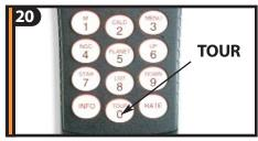
Now that your telescope is properly aligned, you are ready to find your first object. Press the TOUR button on the hand control. The hand control will display a list of objects that are visible for the date and location entered.
