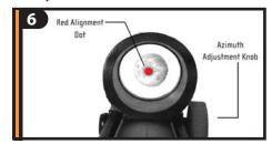
With the object centered in the eyepiece, use the azimuth (right/left) and altitude (up/down) adjustment knobs on the finderscope to place the red alignment dot directly over the centered object.
