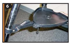
Once grooves are aligned, turn accessory tray until it snaps into clips on each leg brace.
