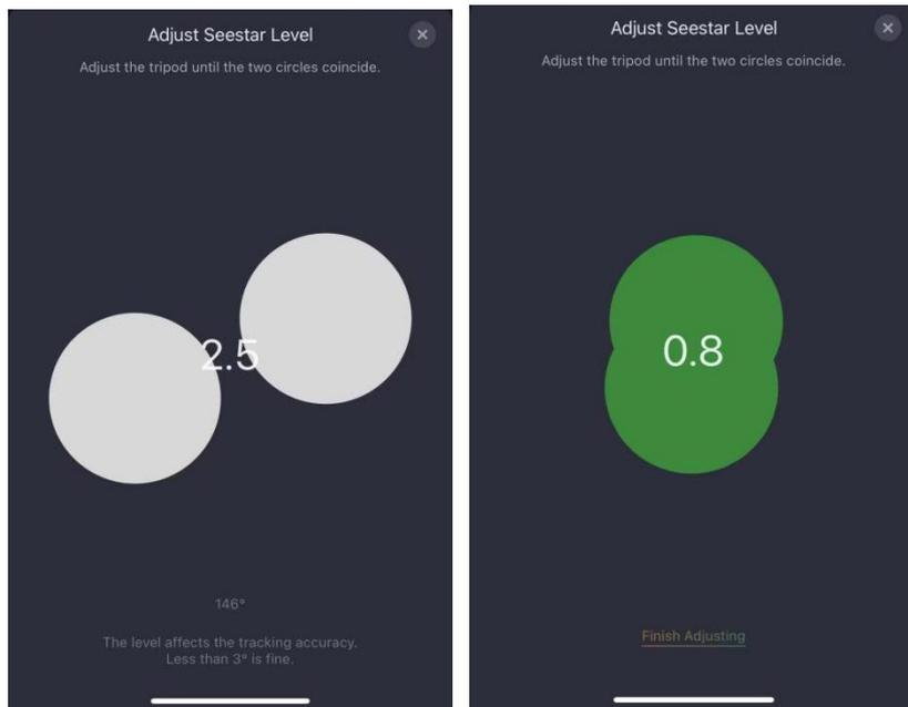
When the device card shows no level, adjust the tripod until the two circles in the picture coincide.
