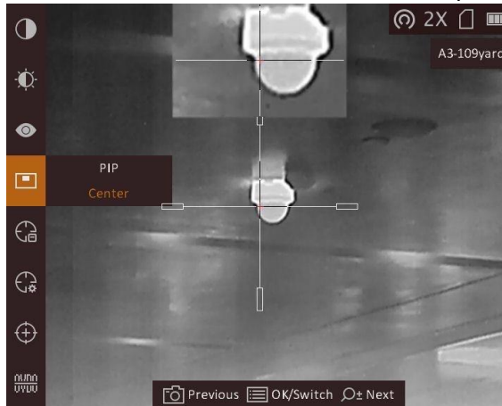
Figure 3-4 Set Picture in Picture Mode
