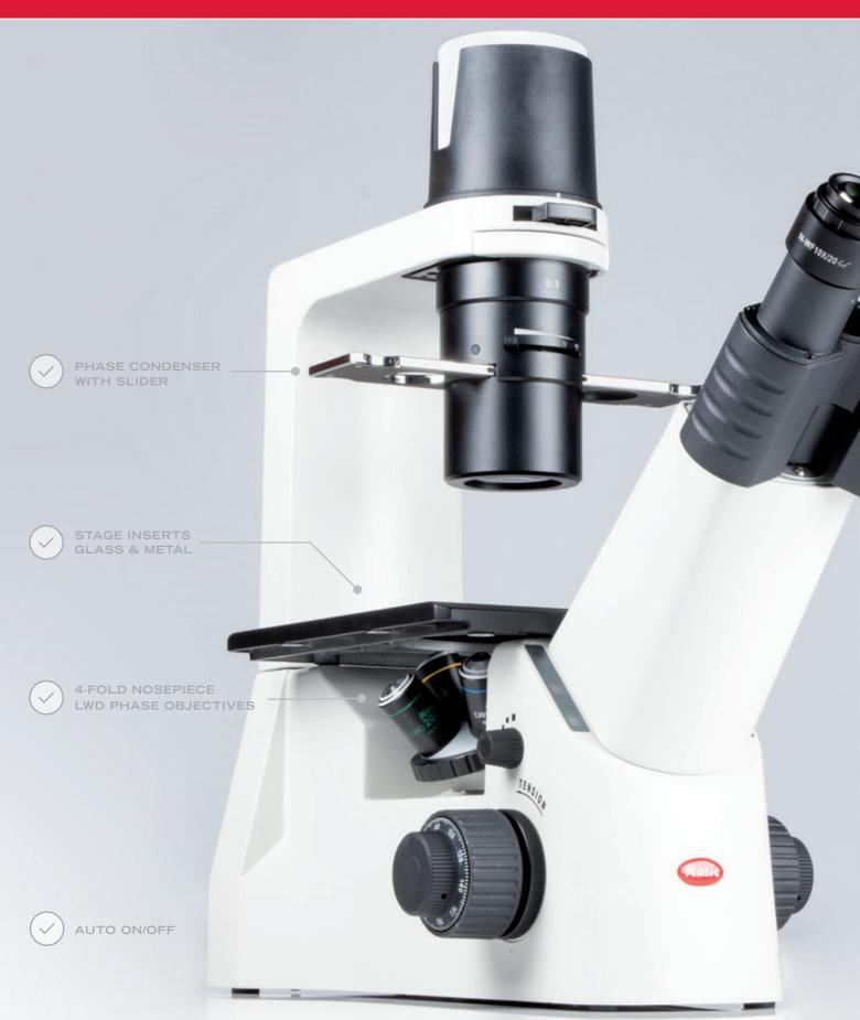
optional 4X Phase objective is dedicated to fast screening. A 40X Phase objective is available too. The AE2000 stand carries a quadruple nosepiece with a precise click stop. Rich illumination power is given by the 30W Halogen light source in a Fixed-Koehler setup, simply interchangeable with 3W LED modules of different color temperatures. The Auto ON/OFF function is a contribution to workplace safety.
