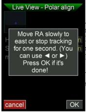
A box pops up. Simply follow the instructions. Your mounts RA axis needs to be slowly moved a little eastwards. You may use the **RIGHT** (or **LEFT**) button on the MGEN-3 to manually send the respective ST4 signal, or you can stop tracking for a few seconds, and then press OK. A little line appears, stretching from the multistar pointing to the pole.
