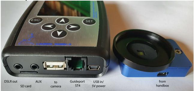
**Power:** The MGEN-3 is powered via the USB port on the bottom right of the handbox (see picture). You may use a normal mobile phone wall adapter, a power bank or a USB port on your PC. The current drawn is typically about 240mA/1.2W.
