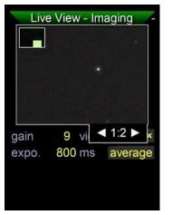
Center on a brighter star. By using **ESC+RIGHT** you can zoom in up to 4:1
