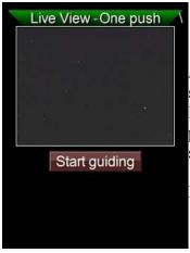
A short press of the **ESC** button turns on the MGEN-3, and after the splash screen the **One push** screen is displayed. What you see here is a live picture from the camera, containing stars. Its a black and white picture because the MGEN-3 camera has a very sensitive monochrome sensor.
