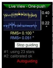
The live picture is then replaced by the guide graph, and at the bottom, Autoguiding is displayed in red blinking letters. You may now start the exposure sequence with your camera.
