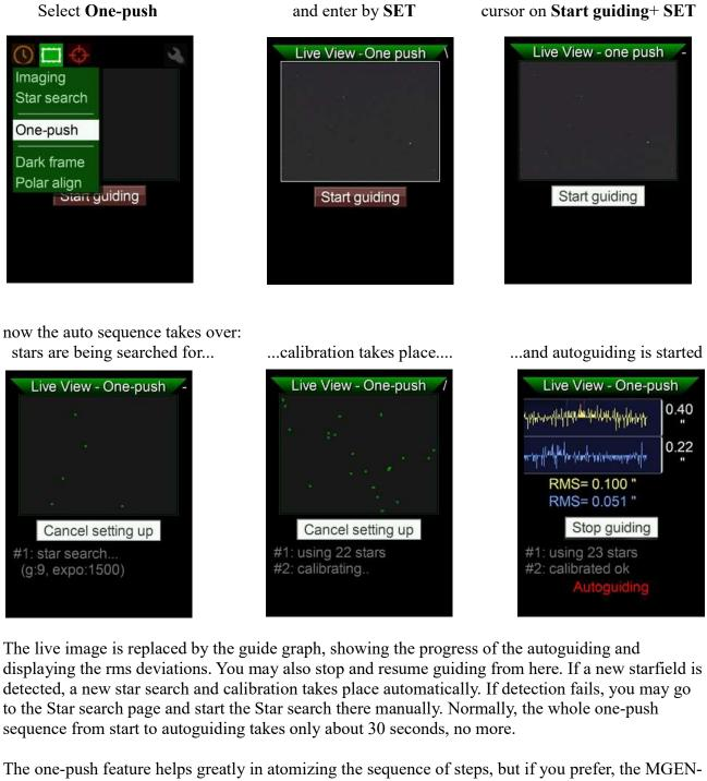
The one-push feature helps greatly in atomizing the sequence of steps, but if you prefer, the MGEN-3 also allows for full manual or semi-manual control. The functions will be explained in detail in following chapters. But before that let's take a look at the DSLR timer and at dithering in order to have everything you need for your astrophotography session clearly understood.
