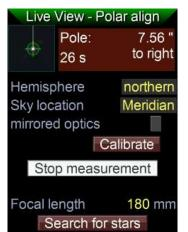
After a few seconds, results appear that are continuously updated as time goes on. The deviation is displayed in size and direction. Wait for about 30 seconds until the number gains stability, stop the measurement and correct the azimuth of your mount. If the pole is to the right, your pole block must also be turned to the right, (clockwise, as seen from above).
