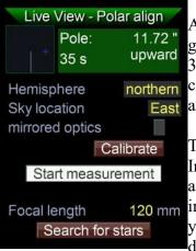
After some seconds results appear that are continuously updated as time goes on. The deviation is displayed in size and direction. Wait for about 30 seconds until the number gains stability, stop the measurement and correct the polar height of your mount. Pole upwards means, your RA axis needs to be set steeper, away from the horizon.
