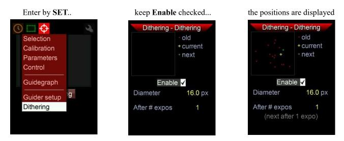
If enabled, the MGEN-3 will shift the guide star automatically a little bit after the specified number of exposures. You can observe the shifting on the active LEDs of the directional buttons when the ST4 output is activated immediately after the DSLR exposure has ended.
