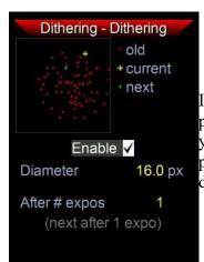
In the box in the upper left there is a graphic display: The previous positions are represented by little red crosses, the actual position by a yellow one, and the next calculated position by a green one. As dithering progresses, a little cloud of red crosses is built up showing the distribution of the points.
