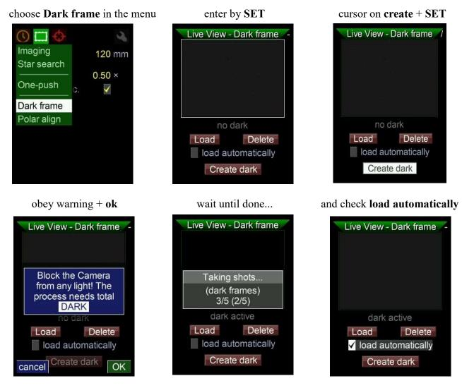
The corrections are applied, **dark active** is displayed and the file is saved onto the SD card. If there is no SD card in the slot, there is a warning, but the corrections remain active until shutdown.
