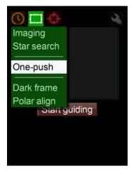
Here you can shift the cursor by pressing the directional buttons UP  $\blacktriangle$  and DOWN  $\lor$ . By LEFT  $\triangleleft$  and RIGHT  $\triangleright$  you can change to other main menus.
