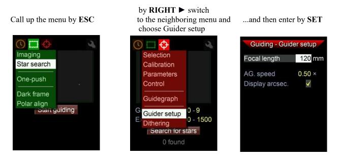
Check if the default values fit or need to be corrected for your setup. A 50mm finder usually has a focal length of 180mm, and a 30mm finder is usually 120mm. A Synta 50mm ED finder has 240mm.
