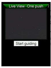
To set the cursor on **Start guiding**, push the **DOWN**  $\checkmark$  directional button, and then press **SET** (from firmware 1.01 the cursor will be on **Start guiding** by default).
