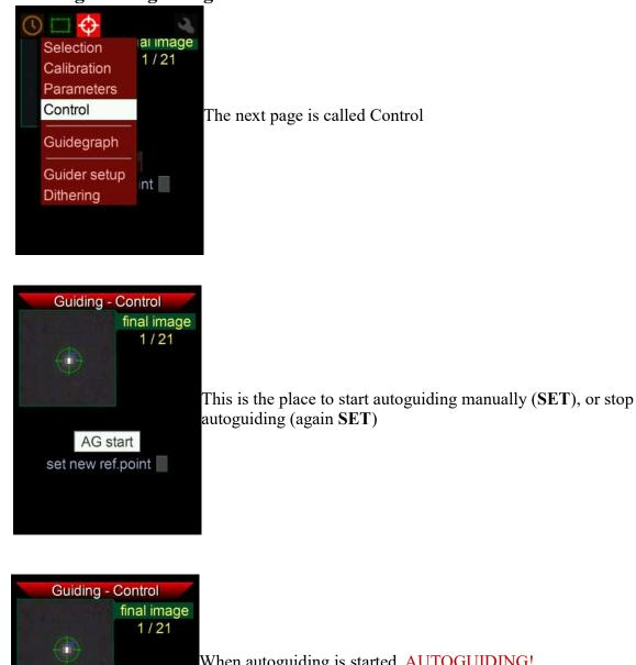
When autoguiding is started, AUTOGUIDING! appears and blinks, and a red cross marks the set point where the star should be kept.
