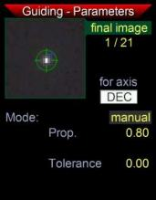
On the DEC page the standard mode is currently **manual** only. The DEC shows neither periodic error nor overtones, but static drifts or erratic movements. So an integral term does not make much sense. Instead, a value of 0.8 for proportional will suit most situations. In the case of overreaction you may lower this value to avoid oscillation of the mount. The tolerance can be left at 0.00, or increased if corrections in the DEC axis need to be dampened. For advanced users only!
