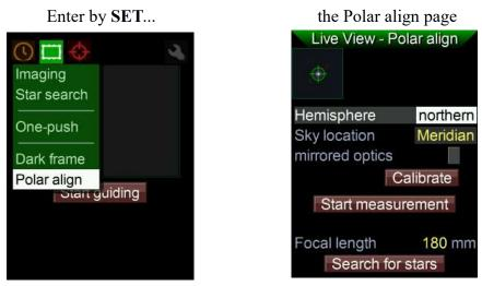
Polar aligning a mount usually is done before autoguiding, so after startup you can switch directly to this page. Set the focal length of your guidescope, if not already done. We recommend to start with a star near the meridian. That helps later on to eliminate the height error as the azimuth is already fine tuned).
