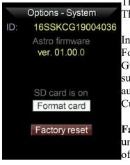
The ID number you need to register your MGEN-3 on the support site. The version number of the currently installed firmware.
