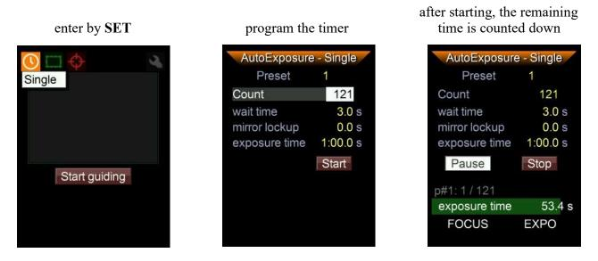
You can pause and restart the exposure sequence at any time. Two signals are sent to the DSLR: First, the focus signal (like half pressing the exposure button) and ESC lights up, then the shutter release signal and SET also lights up. If you want to use mirror lock, you need to activate it in the DSLR. The value 0.0s means no mirror lock. We do not recommend mirror lock with long exposure times. Mirror shake is more of a problem with very short exposures.
