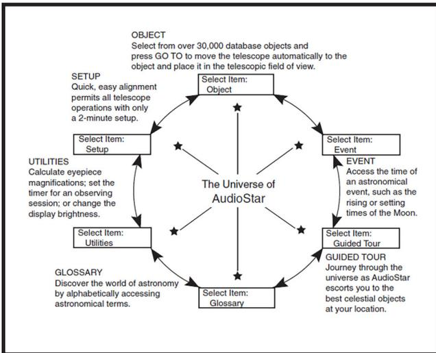
Fig. 8: The AudioStar Universe: The six primary categories listed in the Select Item menu of AudioStar.
