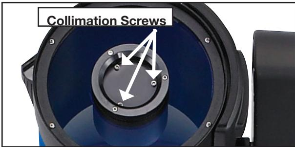
located at the inner surface of the secondary mirror housing.
