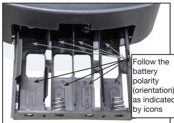
**CAUTION:** Follow battery manufacturer's precautions. Do not install batteries backwards or mix new and used batteries. Do not mix battery types. If these precautions are not followed, batteries may explode, catch fire, or leak. Improperly installed batteries void your Meade warranty. Always remove the batteries if they will not be used for a long period of time.
