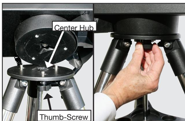
**5** Take the LX65 from its packaging and place the entire telescope onto the top of the tripod head. Rotate the telescope head slowly until you feel the scope register on the center hub of the tripod head. Carefully screw the three attachment thumb-screws on the bottom of the plate to the base of the tripod. Hand tighten the screws so the telescope cannot spin or wobble on the tripod head.
