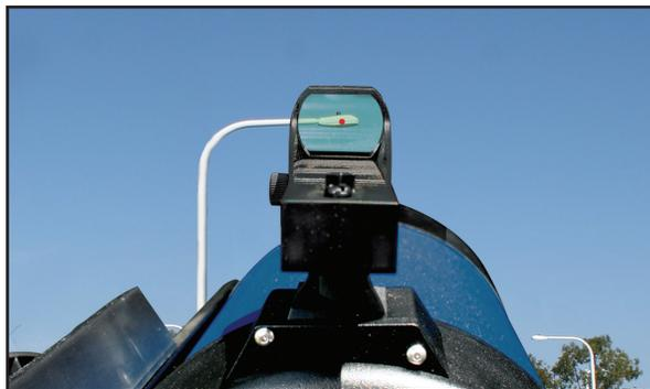
The Red Dot Finder has been aligned at the factory, but you may need to touch-up the alignment from time to time. To do this, look through the eyepiece of your scope and using the hand controller center a distant object. Now turn on the Red Dot Viewfinder and adjust the brightness so you can see the red dot. Look through the sight as pictured above.
