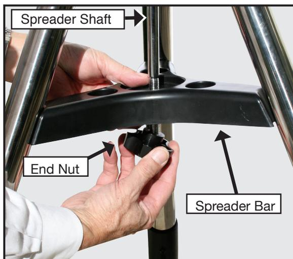
**4** Remove the end nut from the spreader shaft and slide the spreader in between the telescope legs. Attach the end nut and hand tighten until the telescope legs are held snugly in the most spread position. Position the tripod where you want the telescope to be and check that the top of the tripod is approximately level.
