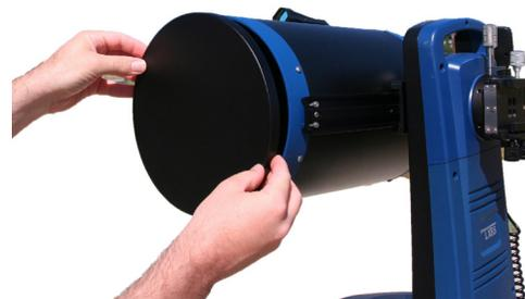
On the optical tube, remove the dust cap from the rear cell of the telescope. Thread the 1.25" eyepiece holder onto the rear cell thread. Slide the diagonal mirror into the eyepiece holder and lock in place by turning the thumbscrew to a firm feel. Place the Super Plössl 26mm eyepiece into the diagonal mirror and tighten the diagonal mirror thumbscrew to a firm feel only.
