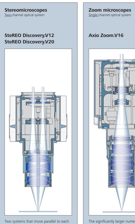
two systems that move parallel to each other feature a common main objective. The circumferential pairs of light rays produce a convergence, or stereo, angle that creates the impression of a 3D image. The significantly larger numerical aperture of the widened optical channel results in a higher level of resolution and brighter fluorescence in equivalent fields of view.
