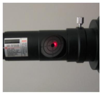
Figure 22:The primary mirror is not yet collimated.
