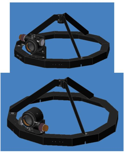
Figure 11: Attach the focuser to the L bracket
