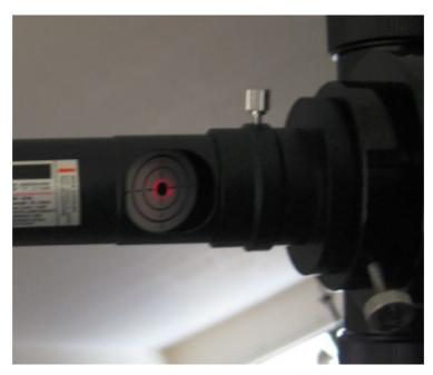
Figure 23:The primary mirror is collimated by laser collimator.
