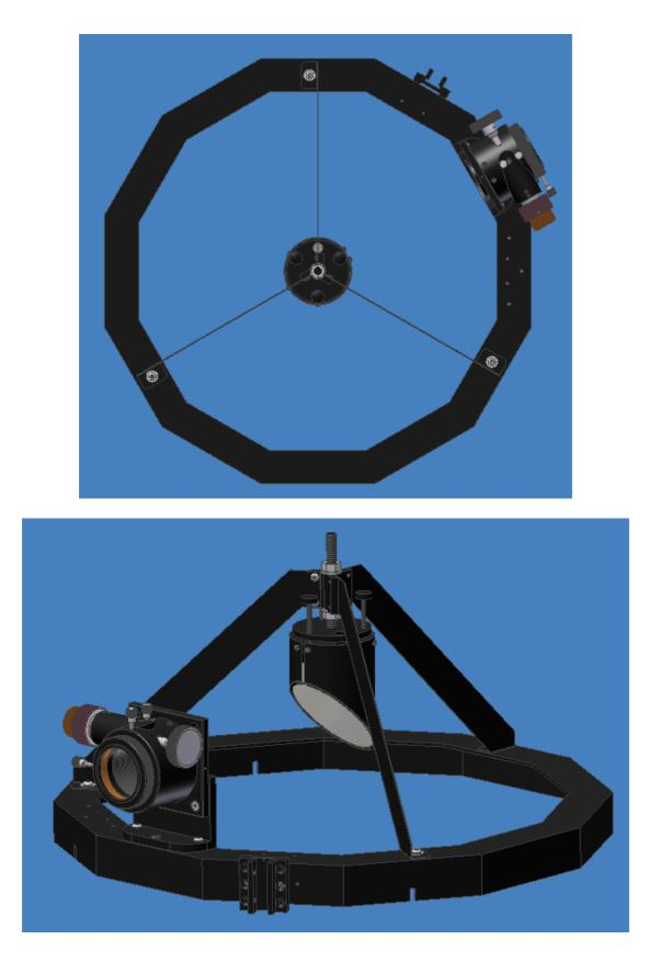
Figure 12: Attach the secondary holder with the secondary mirror
