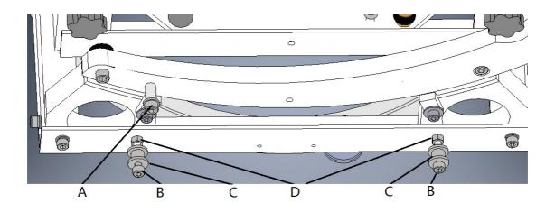
M6 plastic wrapped anchor screw (A) M5 x 40 screws (B), rollers (C), and locking nuts.
