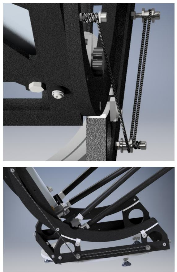
UP12 rubber band based virtual counter weight system
