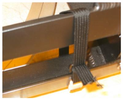
Tie the mirror box to the rocker with nylon strips for the safety
