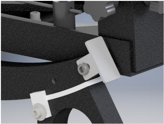
The Bottom ALT bearing limit block
