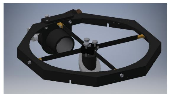
Attach the secondary mirror holder to the central bolt
