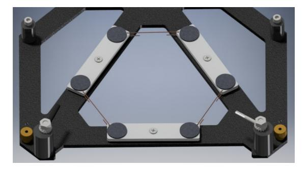
First bend the three brass wires into U shape, with the center portion about 64 mm (a bit longer is OK, but all three should be the same length, as much as possible).
