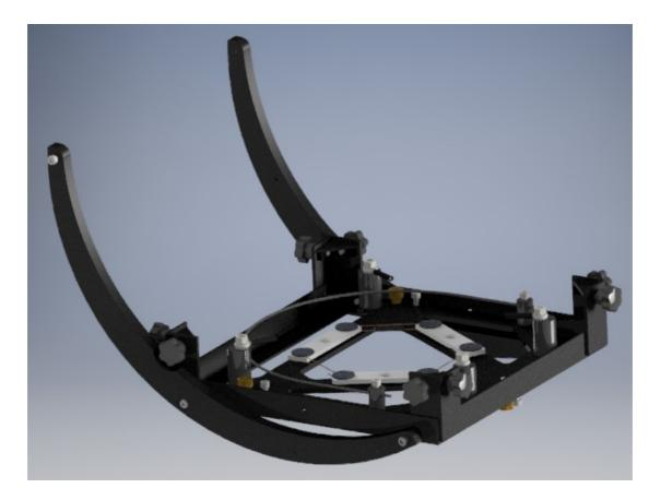
• Then rest the mirror box on the Rocker, and install the two ALT bearing limit blocks on one of the bearing.
