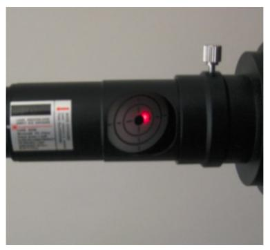
Figure 5: The primary mirror is not yet collimated.
