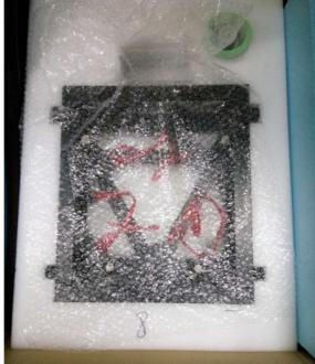
The Mirror Box Protection Ring is bolted to the mirror box by the knobs. The secondary mirror safe container is at the up right corner in the above picture. The protection ring is not used to assemble the scope, and is only used to pack the scope.
