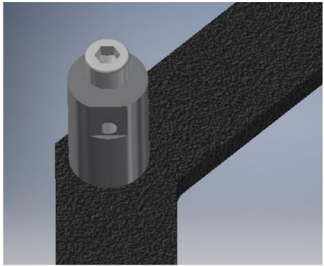
The stainless steel cable anchor post and the top locking screw
