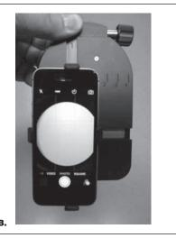
**Figure 1.** Removing the bumper or case from your smartphone may avoid a constricted field of view as in **A**. With case or bumper removed the image will fill more of the phone's screen, as in **B**.
