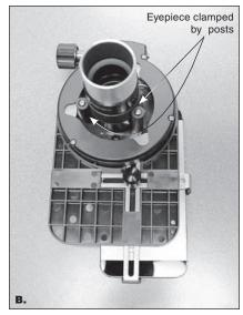
**Figure 5. A)** Place the eyepiece upside down on the SteadyPix as shown, then **B)** rotate the eyepiece clamp knob clockwise until the three clamp posts grip the eyepiece housing firmly.
