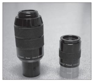
**Figure 2.** Examples of two eyepieces with housing diameters that are compatible with the SteadyPix EZ. The 25mm Sirius PlossI (right) has a housing diameter of 35mm; the 3mm Edge-On Planetary eyepiece has a housing diameter of 45.5mm. Both eyepieces are shown with their rubber eyecups removed.
