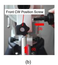
Figure 11. Install counterweight shaft
