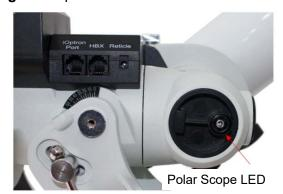
Figure 19. Polar Scope LED
