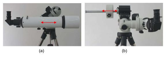
Figure 15. Balance along R.A. axis (a) and DEC axis (b)
