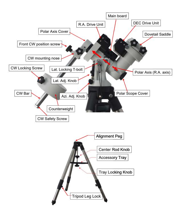
Figure 1. CEM25 assembly terms (mount and tripod)
