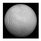
Another effect present in CCD imaging of monochrome light of Hydrogen Alpha or Calcium H is the interference pattern - or Newton's Rings. The effect is similar to interference testing of an optical surface between two flat surfaces. The sensor and cover slip cause a small interferometer inside the camera and cause a Newton's Ring moire' pattern. The CCD chip must be tilted to a minor degree to prevent this pattern. Recent
