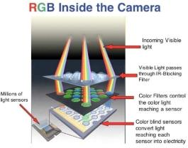
(Canon and Nikon) use an IR blocking filter which greatly reduces the transmission of Hydrogen Alpha light. DSLR cameras without this IR blocking filter will have better sensitivity imaging in Hydrogen Alpha.
