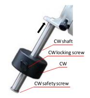
Figure 6. CW shaft and CW
