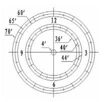
are 2 groups, 6 concentric circles marked from 36' to 44' and 60' to 70', respectively. The 36' to 44' concentric circles are used for polar alignment in the northern
