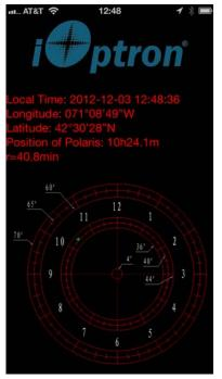
Adjust the mount in latitude and azimuth direction to place Polaris in the same position on the Polar Scope Dial as indicated on your iPhone/iPad screen. In this case. the Polaris will be located at a radius of 40.8' and an angle of 10 hour 24.1 minute.
