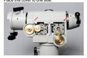
3. It is recommended to work on 1 axis drive at a time. Identify the declination motor connector and carefully un-plug the motor lead from the circuit board. Note the route of the motor wires. It may be necessary to un-twist the motor wires from other cables.
