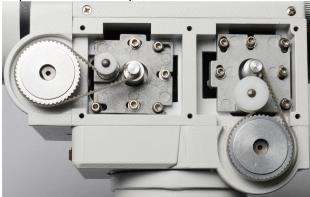
Once the RA belt has been fitted it is now a good opportunity the check the drive operation. Power up the mount and slew the axis drives using your handset.
