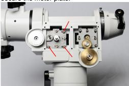
14. For the Dec axis, place the small idler on to the 5mm pin with the wider edge of the idler uppermost. (The larger idler fits to the RA axis.)
