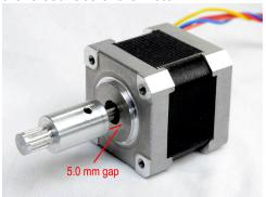
9. Fit the 5.0mm pin in to the motor plate and tighten the 2 x m4 grubscrews. The top of the pin should be level with the top of the pulley.
