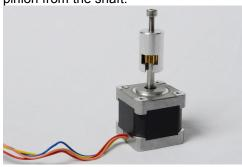
8. Fit the 9 tooth pulley on to the motor shaft and gently 'nip' the 2 x m3 grub screws. Do not over tighten. A 5.5mm gap will be between the pulley and the raised face of the motor.
