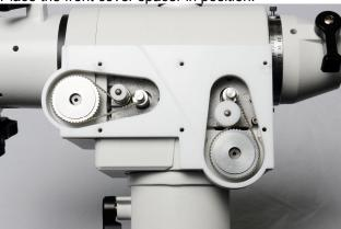
Fit the front cover in position on the spacer and using 6x M3x16 socket head screws, gently tighten down.
