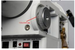
13. Replace the motor in to the mount housing carefully feeding the motor wires back to the circuit board. Carefully check the wiring does not interfere or touch the declination shaft. Replace 3 x screws to secure the motor plate.
