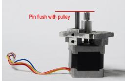
10. Replace the screws holding the motor plate and motor. Position the motor wires as noted in step 6.
