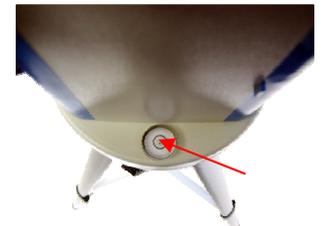
If the bubble does not stay inside the small circle, you may need to calibrate the level by make sure it stays at the same position while rotating the mount. Mark the new bubble position as a calibrated center position. It is also recommended to use an additional levelers (such as a torpedo leveler) to assure precise leveling.
