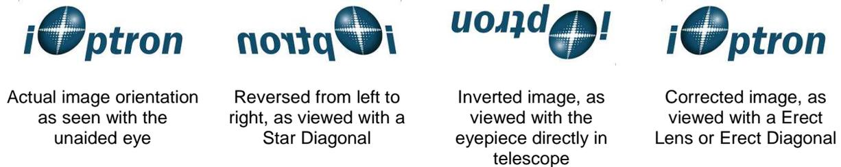
For terrestrial observation, such as land mark or bird viewing, you can buy an optional 45° Erect Diagonal to have a correct image from your eyepiece.
