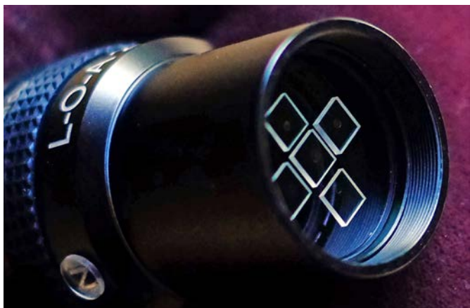
This glass array, which Denkmeier attached to one of the eyepiece's field lenses, creates the 3-D effect.
