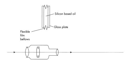
When the binocular moves, the angle between the plates of the vari-angle prism changes to compensate.
