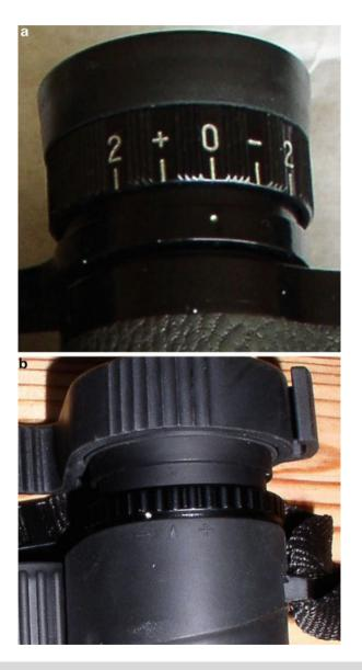
Fig. 2.29 Right eyepiece diopter adjustment. (a) Porro prism. (b) Roof prism
